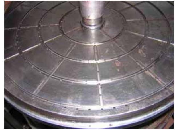
15. Press plate with holes to allow butter removal
