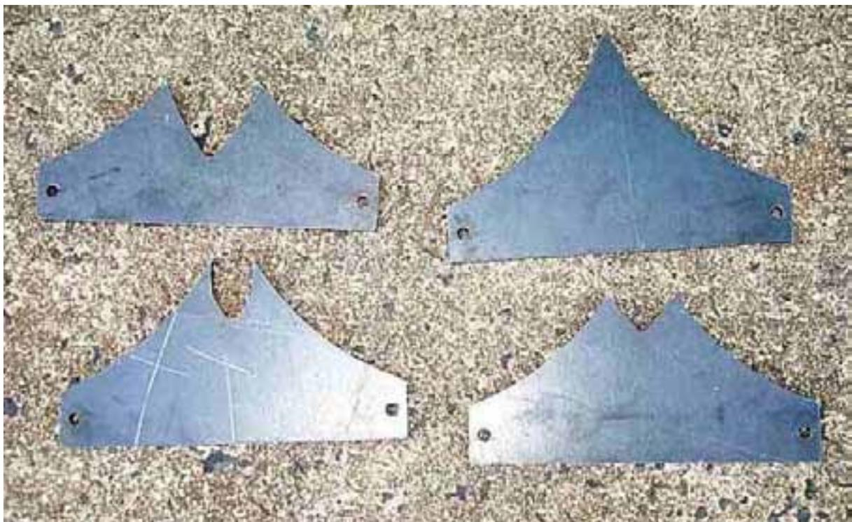
**Figure 5.14** Alternative splitter plate shapes.
