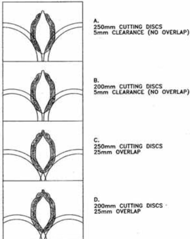
**Figure 5.17 Area of cut achieved (shaded) using four alternative cutting disc configurations.**
