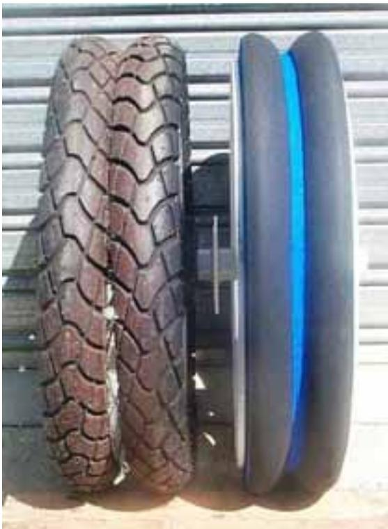
**Figure 5.19 Profile comparisons of original pneumatic tyres (left) and custom manufactured EVA ‘tyres’ (right).**
