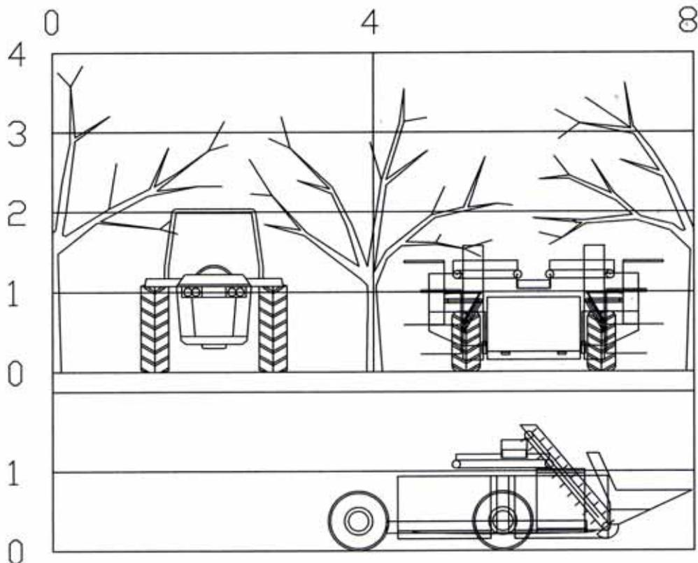
**Figure 7.20 Self-propelled cocoa harvest aid. Note the orchard tractor is inserted for reference only.**
