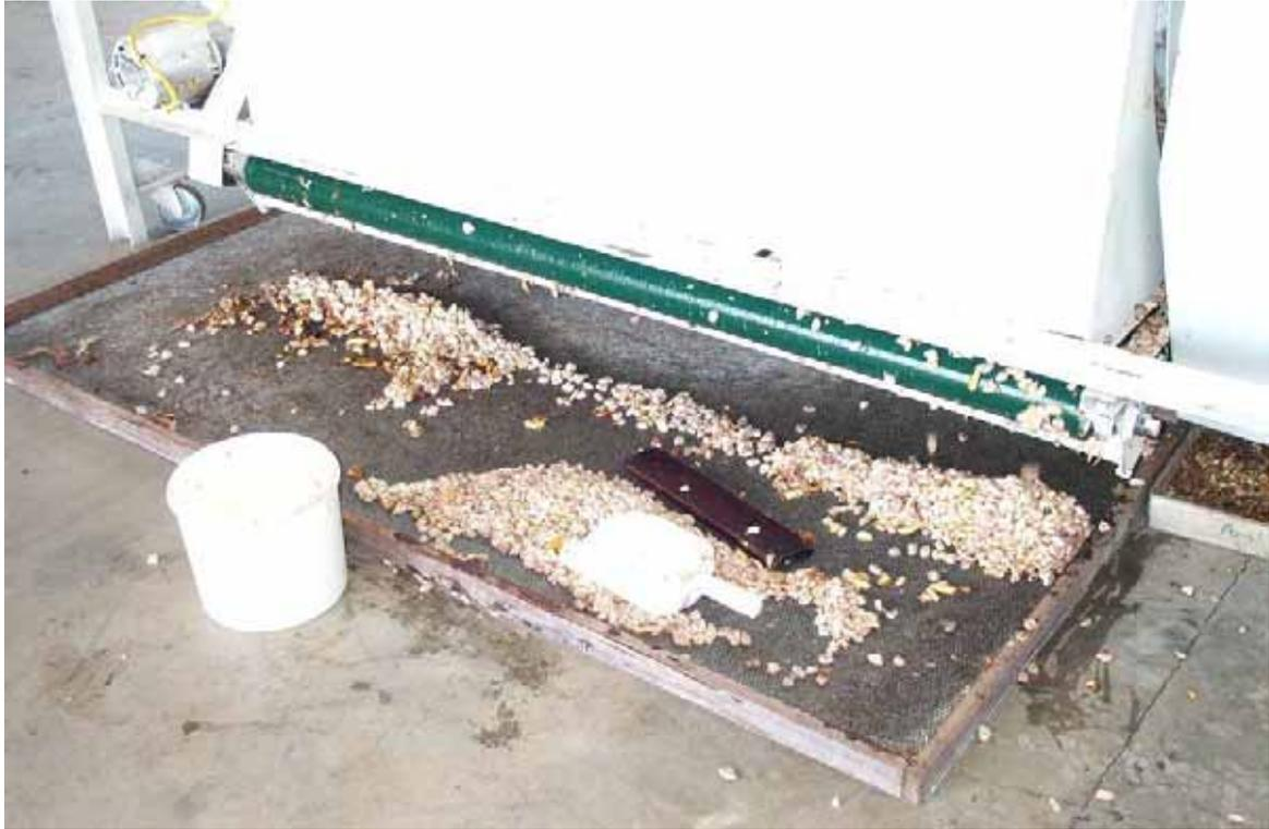
Figure 5.26 NACDA bean separator showing wet bean conveyor belt.
