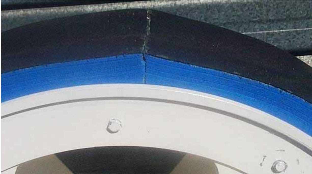
**Figure 5.21 Deformation caused by glued join of EVA tyre.**
