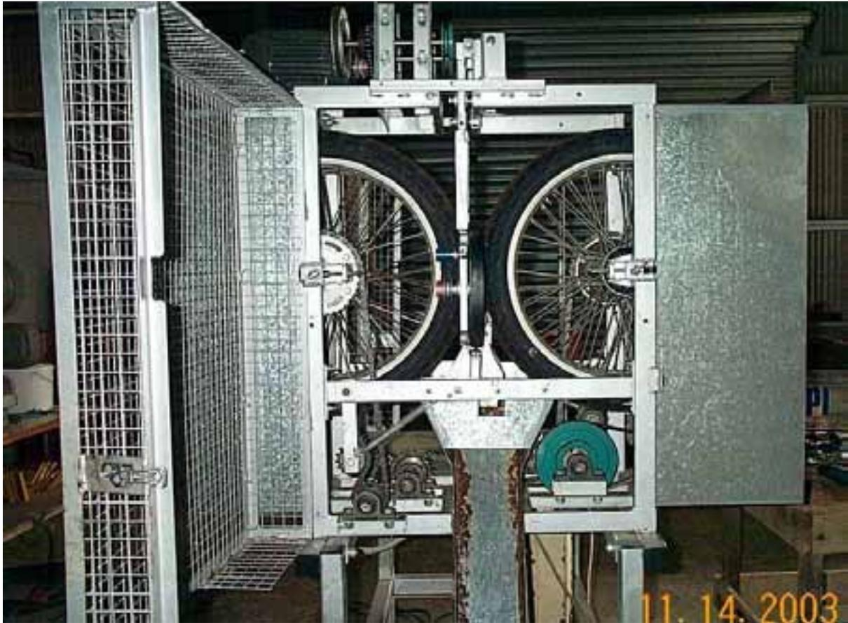
**Figure 5.15 Overview of redesigned pod splitter.**
