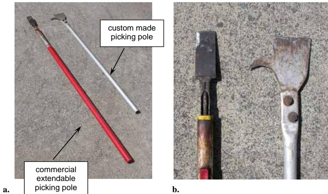
**Figure 7.14 a. Picking poles used for harvesting high cocoa pods (custom made pole proved unsuitable). b. Close up of cutting heads.**
