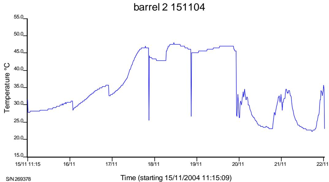
**Figure 6.10** Barrel fermentation in warmed room.
