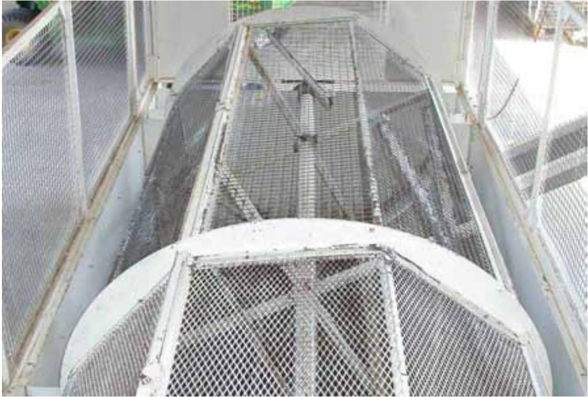
**Figure 5.25 NACDA bean separator showing two-stage demountable screens.**
