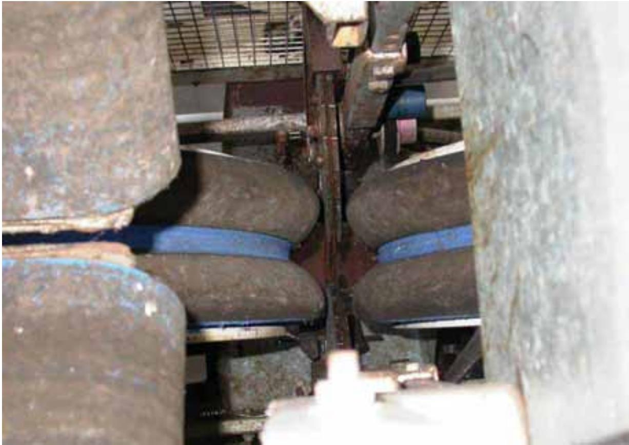
**Figure 5.20** EVA 'tyres' as fitted to the pod splitter (view from above).
