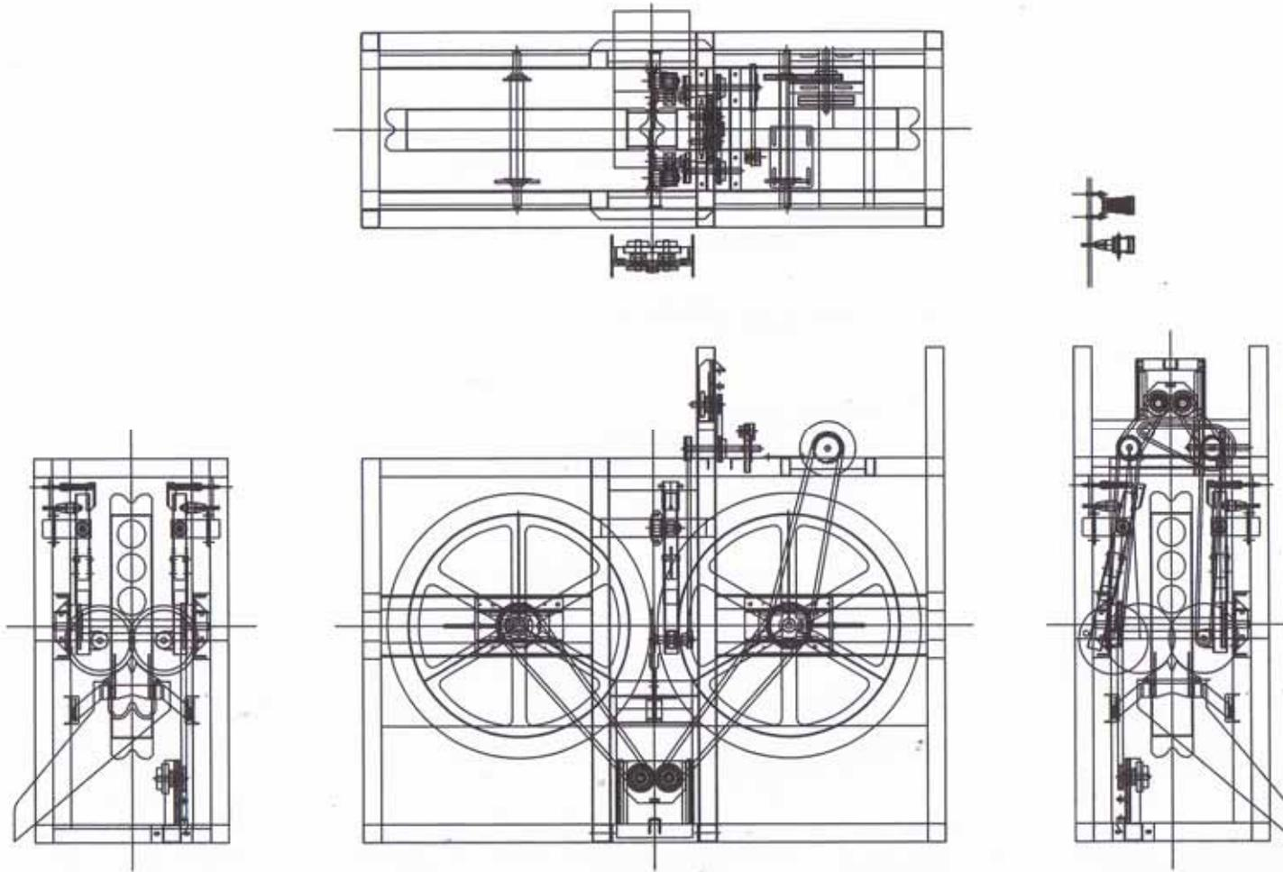
Figure 5.22 Conceptual drawings of NACDA Mark II pod splitter
