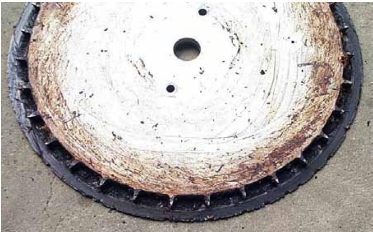
**Figure 5.13 Spiked backing plate on cutting wheel.**
