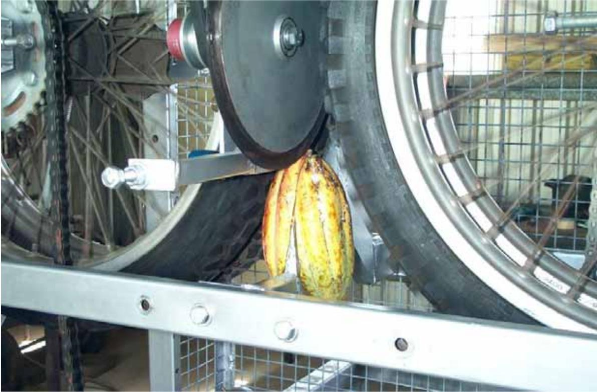
Figure 5.11 Pod being split by arrowhead plate.
