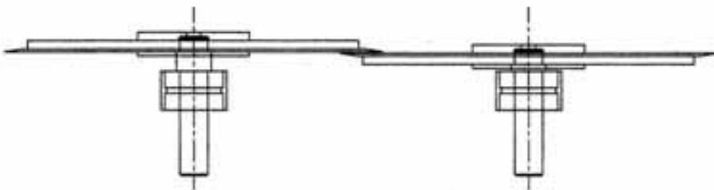
**Figure 5.16 Configuration of overlapped cutting discs (plan view).**
