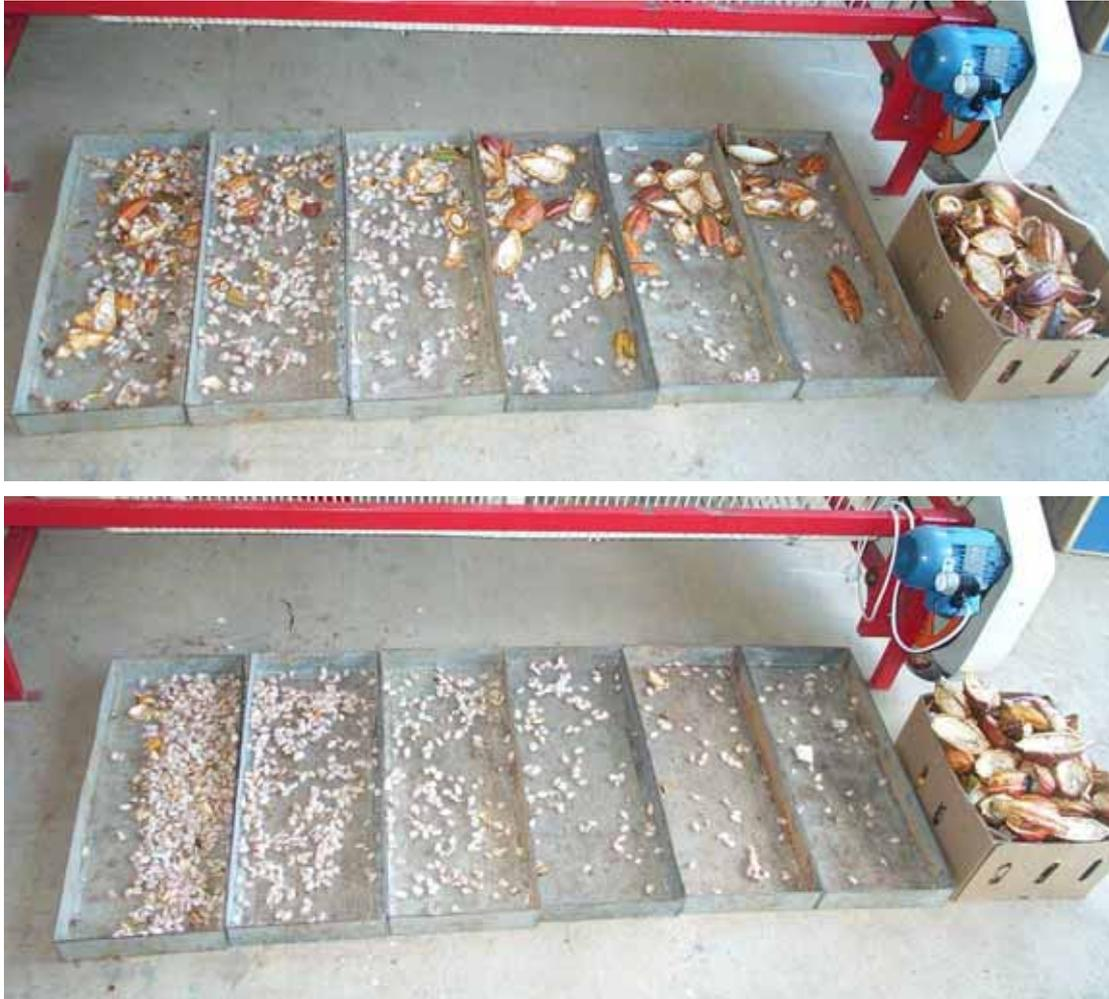
Figure 5.7 Material samples post-pod splitting by Brazilian pod splitter (top) and NACDA pod splitter (bottom).
