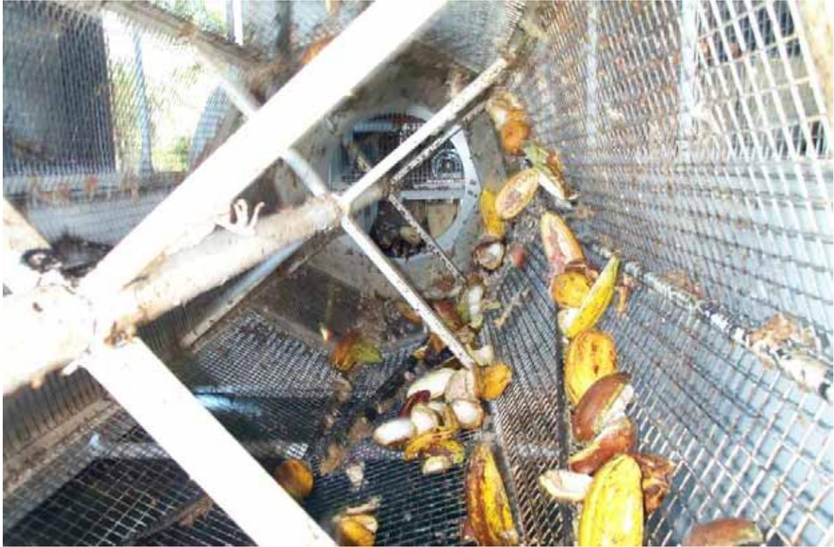
**Figure 5.24 NACDA bean separator in operation.**
