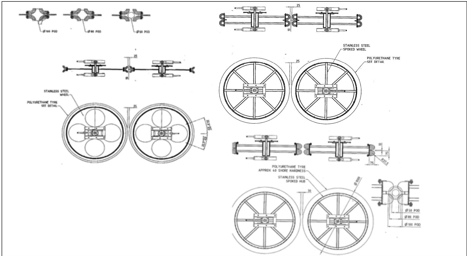
Figure 5.18 Proposed alternative 'tyre' arrangements based on moulded urethane construction.
