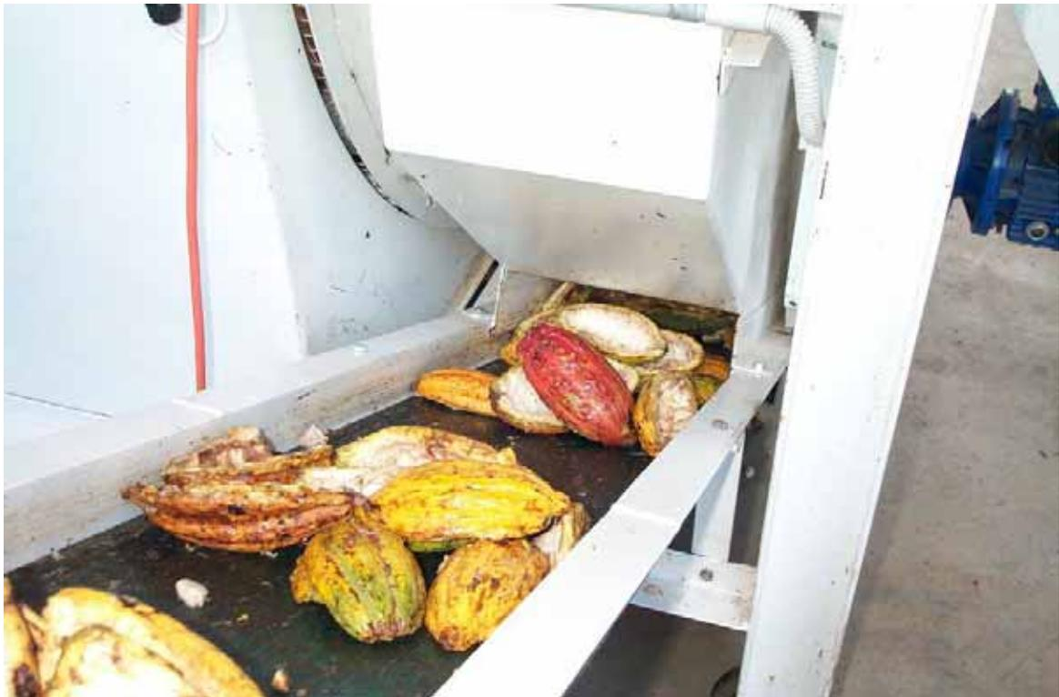
Figure 5.27 NACDA bean separator showing pod husk waste elevator.
