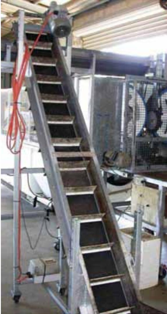
**Figure 5.29 Pod elevator.**
