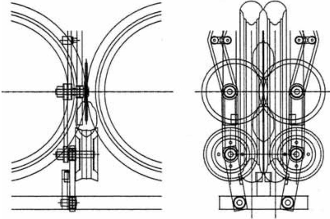
Figure 5.8 Schematic view of crusher wheel arrangement.
