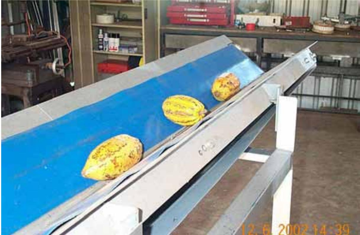
**Figure 5.28 Pods on prototype pod conveyor.**
