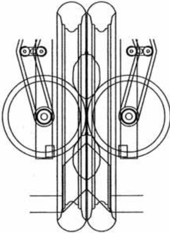
**Figure 5.10 Set-up of arrowhead splitter.**
