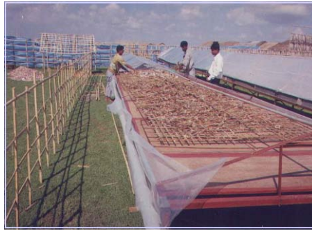
Figure 4.2. Drying of fish in solar tunnel drier
