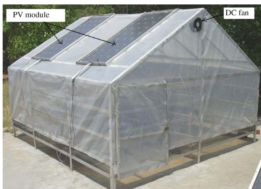
Figure 6.17. Hybrid photovoltaic-thermal (PV/T) integrated greenhouse dryer ( Barnwal and Tiwari 2008 )
